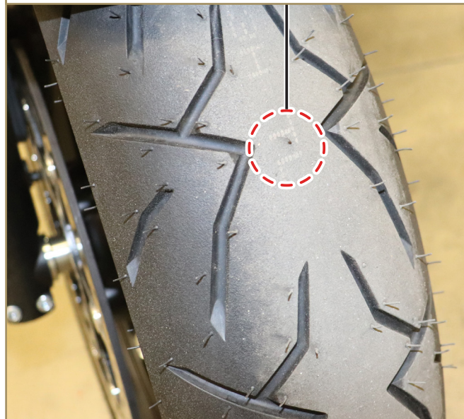
Surface warning mark
